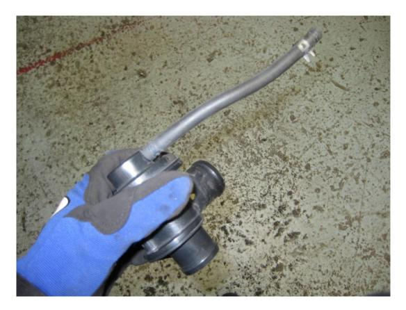
6. Remove the spring clamps from the vacuum line and place them onto the new silicon vacuum line supplied, about 50mm from the ends. Push the new vacuum line onto the port on the engine, and secure it with the spring clamp. Leave the other end disconnected at the moment.
