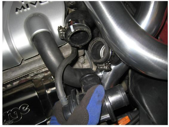
4. ....then locate where the vaccum line joins the engine, and squeeze the spring clamp with your needle nose pliers to loosen it, and pull it back down the vacuum line.
