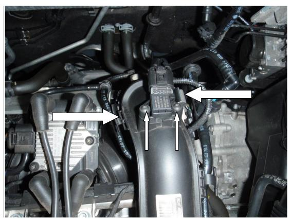
4. Remove the engine lifting eye as arrowed below.
