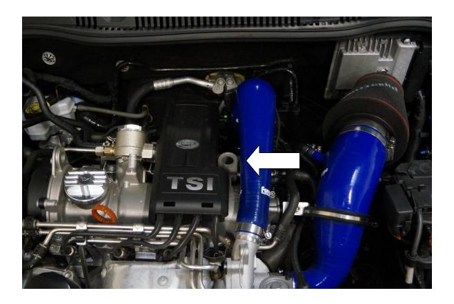
4. Remove the rubber O ring from the plastic boost pipe and insert into the alloy dump valve adaptor
