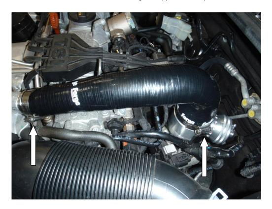
8. Unclip the second map sensor from the inlet manifold and insert the alloy take off.9. Insert the map sensor into the alloy take off and secure using the provided self tapping screws.
