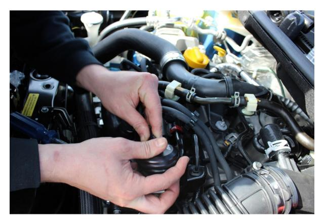
9. An extra half a metre of vacuum hose is included in the atmospheric valve kit. Replace the vacuum hose if the OEM hose is too short (this can vary from vehicle to vehicle).
