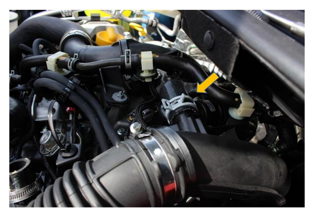
8. Fit the Forge atmospheric valve into position.
