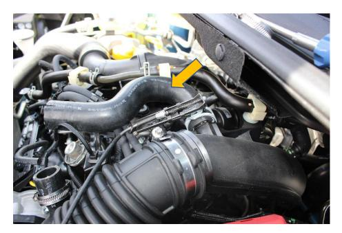
7. Fit the supplied blanking hose using the original clamp as pictured below.
