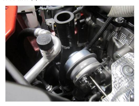
7. Locate the actuator and remove the M6 nut shown by the arrow in the picture below with the use of a 10mm spanner or rachet drive.
