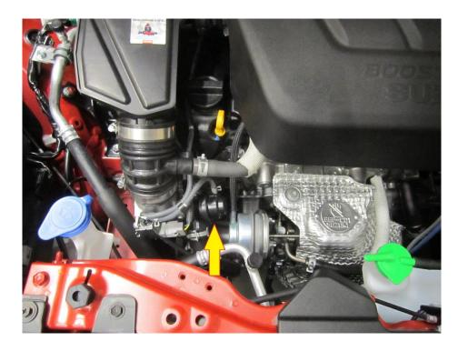
2. Unclip the vacuum hose clamp at the top of the valve then remove the vacuum hose from the valve, follow the hose to where it connects to the solenoid and remove it completely as you will be fitting a new hose later in the installation. There is an M6 fastener attaching the valve to the turbo elbow, undo this bolt to free the valve.
