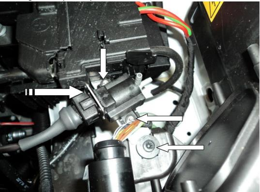
8. You will now need to fit the vacuum hose between the valve and solenoid.
