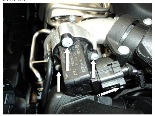
2. At the rear of the engine, on top of the inlet manifold, you will find the map sensor. Undo the two T20 Torx bolts and pull upwards on the sensor, removing it (leave the plug connected).
