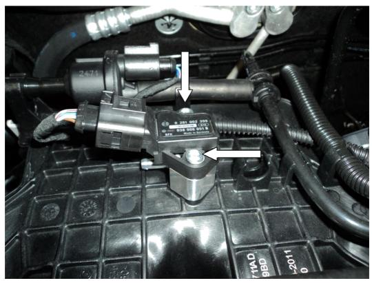
4. Fit the new Forge valve onto the turbo with the existing T30 torx bolts where the OEM valve was situated. Make sure the orientation of the vacuum take off pipes are the same as in the picture below.
