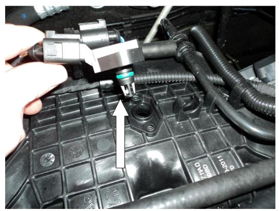
3. Push the new Forge aluminium vacuum take off block onto the bottom of the sensor, (this can be a tight fit), making sure the vacuum take off pipe is facing to the left. Refit this back into the inlet manifold using the Phillip's headed self-tapping screws provided.
