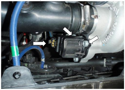
4. Bolt the solenoid onto the bracket supplied in the kit. On the radiator pack you will see a bolt protruding, bolt the bracket onto the radiator pack with the M6 nut supplied in the kit as shown below. Bolt on the dump valve with the bolts that were removed from the stock dump valve.
