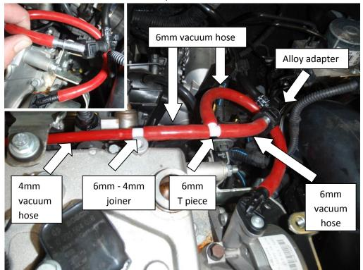
6. Pass the 4mm vacuum hose under the wiring etc at the back of the engine. Place around the dip stick then straight down to the solenoid.
