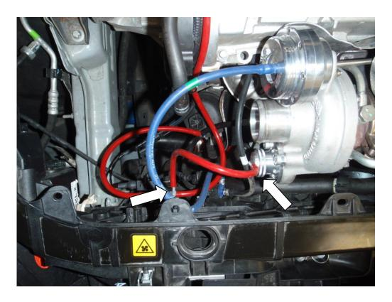
11. Using the zip ties supplied secure all of the installed vacuum hoses and trim off excess refit the air filter and engine cover. Installation is complete!
