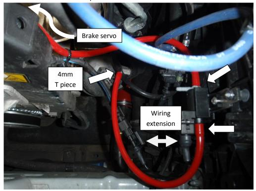
10. Connect another short length of 4mm silicon vacuum hose from the solenoid to the dump valve.
