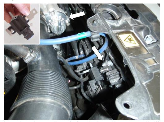
5. Remove the engine cover, close to the throttle body you will see a vacuum take off for the brake servo. Disconnect the vacuum take off cut the appropriate lengths of 6mm vacuum hose and join together with the 6mm T piece. Also join the 6mm reducing to 4mm coupler as shown below, with the aluminium adapter reconnect the vacuum take off.
