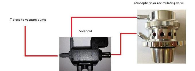
7. Connect the plug on the supplied harness to the solenoid, and then using the supplied red wire taps, tap into the two wires on the vehicle such that the red/green Mercedes wire goes to the red wire on the Forge harness, and the black wire on the Forge harness goes to the other Mercedes wire (colour may vary).
