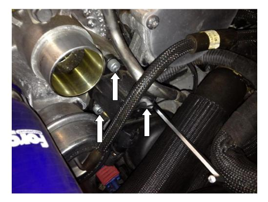
5. Remove your Forge valve from the box and insert the o-rings supplied into the bottom face of the valve, then bolt the valve to the turbo using the bolts supplied. Note the valve will only fit one way round, meaning the vacuum port on the base of the valve points DOWN (the port on the top of the valve can be pointed in any direction).
