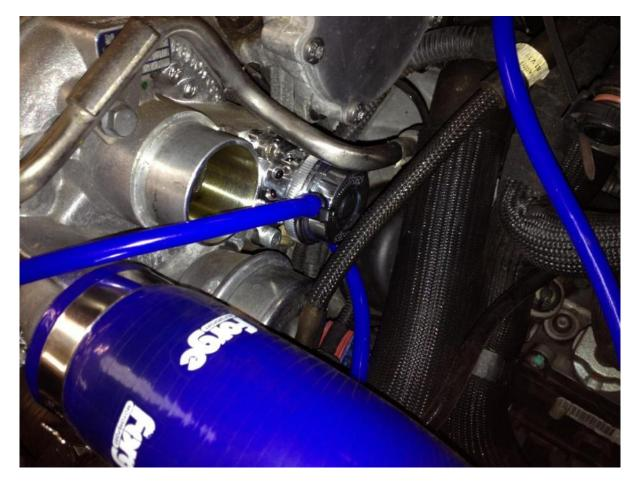
Tools needed: 5mm allen key Hose clamp driver Wire cutters 10mm socket and suitable ratchet 1. Open the bonnet and undo the hose clamps on the hose between the intake and turbo inlet. Squeeze the fittings to release them from the breather on the cam cover and the fitting on the underside of the inlet hose, then remove the hose from the car (Forge inlet hose shown FMINDRCZ). Undo the 10mm bolt holding the cold air feed to the airbox.
