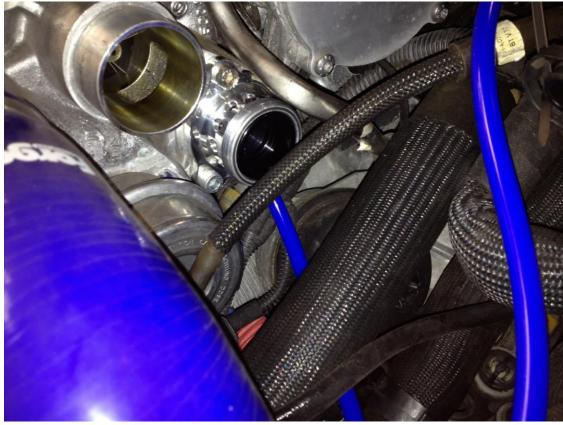
10. Replace the top of the valve (if removed) and screw the top down such that the vacuum outlet on the top of the valve is pointing downwards at an angle as shown (to keep things neat). Use the silicon vacuum hose left over to connect this port on the dump valve to the last port on the solenoid which is the VERTICAL plastic port. Use the cable ties provided to secure all the ends of the vacuum lines to the solenoid, valve and tee piece on the vacuum pump.
