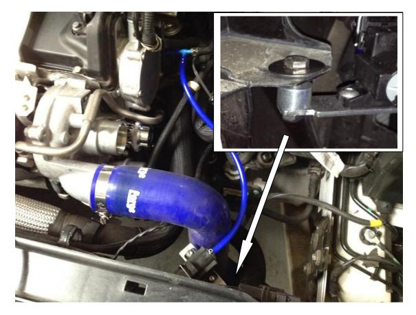
9. Connect a vacuum hose to the LOWER port on the dump valve. You may find it easier to unscrew and remove the top of the valve to do this. If you do, make sure you catch the spring as you unscrew the top. Route this vaccum hose to the REAR METAL port on the solenoid, cut the hose to length and fit.
