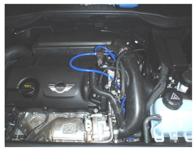
Tools Needed: 7mm Clamp Driver 10mm Spanner/Socket 8mm Socket 5mm Allen key 3mm Allen key 1. Open the bonnet and using a 7mm hose clamp driver, undo the 2 hose clamps on each end of the intake pipe, once these are loosened squeeze the 2 tabs together using your fingers on the oil breather pipe and remove the pipe along with the air intake pipe.
