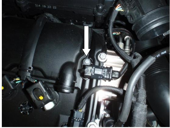
7. Now install the solenoid provided along with the M6 bolt and spacer making sure orientation is correct, putting the spacer over the hole first then the bracket and then the bolt.
