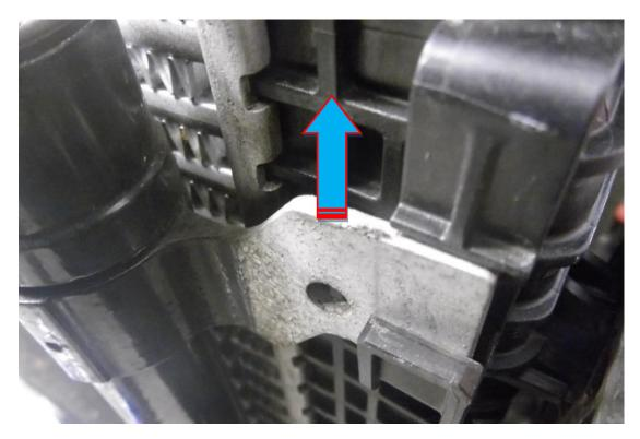
25. The radiator and intercooler are attached to the radiator pack frame with two plastic sprung clips (one per side), using pliers break the anchoring points off to free the radiator and intercooler.
