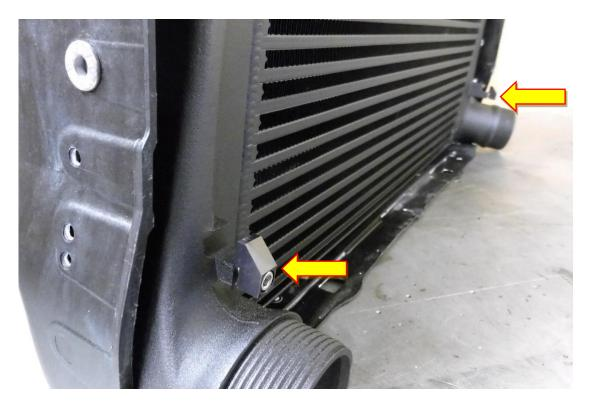
**32**. Fit the radiator to the intercooler, make sure the lower locating pegs of the radiator are seated inside the clamps, push the upper retaining clips into position to secure the radiator. Using a 6mm Allen tighten the clamp.
