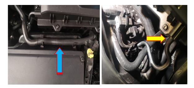
6. The airbox is located by rubber grommets on three pins. Rock the airbox left to right while pulling in an upwards motion to remove it. You can now remove the front air ducting highlighted with the yellow arrow.
