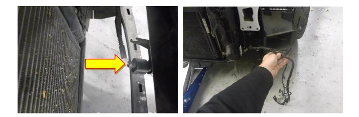
21. Using aT30 Torx and drive remove X4 M6 fasteners (X2 per side) that attach the crash bar to the radiator pack.
