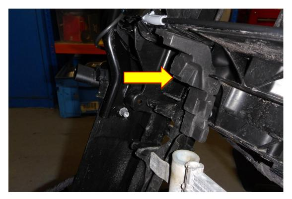
27. Using a flat blade screwdriver or trim tool, push both retaining clips down to separate the radiator from the intercooler. Once parted lift the radiator upwards from the intercooler to completely remove the radiator from the intercooler.
