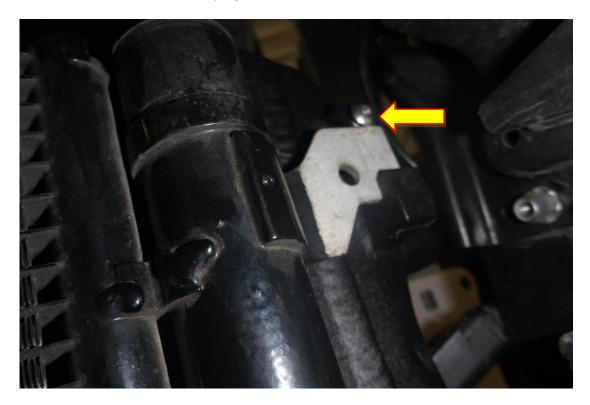
**34**. Using a Pozi drive screwdriver secure the intercooler into the radiator pack frame. There is a hole in the centre where the old bracket located. Using the two screws provided, screw these into the new brackets on your intercooler and tighten both sides.
