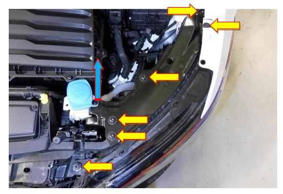
If your vehicle is not equipped with a gas bonnet strut, for the following steps you need to find something suitable to support the bonnet temporarily. We removed the bonnet stay and relocated it under the coolant expansion tank. Un-attach the bonnet release cable from the headlight bracket.
