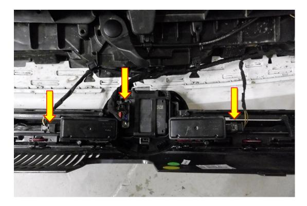
4. Using a T25 Torx and drive remove the x2 M5 fasteners that hold on the airbox duct and use a hose clamp removal tool to loosen the inlet hose from the air box.
