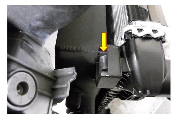
**33**. Tilt the complete radiator pack slightly away for you and fit the air conditioning condenser to the intercooler mounting hooks. Using a 3mm Allen key secure the condenser with the supplied M5 fastener to the threaded hole located above the top right bracket.
