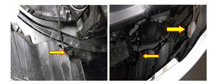
Once all plugs are disconnected you can now remove the bumper completely.
