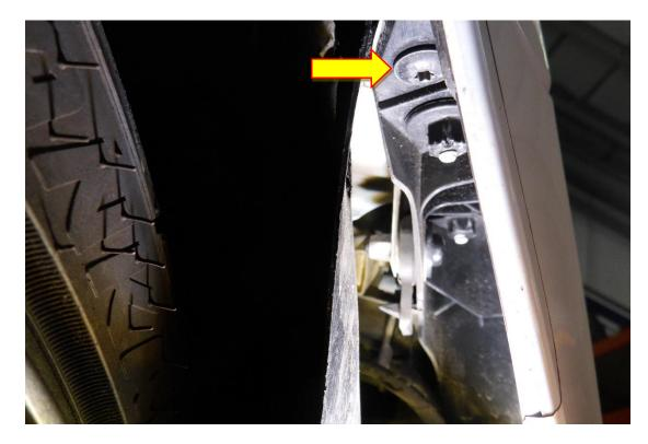
**10**. Using a T25 Torx and drive remove the x9 M5 fasteners attaching the bottom of the bumper.
