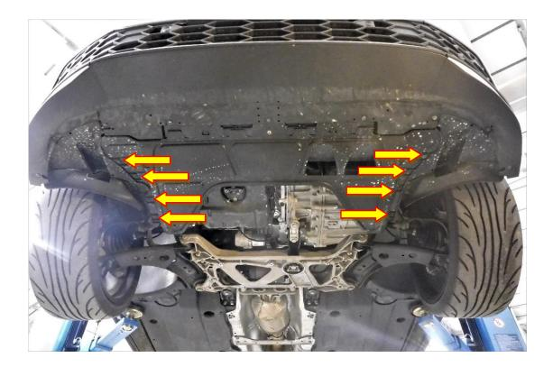
12. Pull sharply on the sides of the bumper to release them from the vehicle. You will now be able to release the bumper from the vehicle but not fully, but enough to allow access to unplug the fog lights and parking sensor connector.
