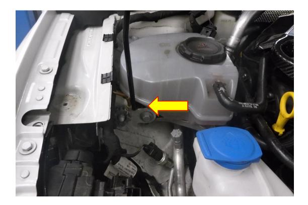
14. Using a 10mm socket and ratchet remove the x2 nuts attaching the plastic bumper support to the wing. Using a T30 Torx and drive remove the M6 fastener.
