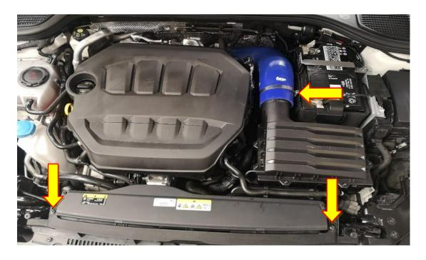
5. Unclip the coolant hose from the front of the airbox lid. Disconnect the vacuum hose attached to the front left of the airbox.
