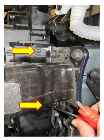
22. Using a 17mm socket and ratchet remove X8 M10 fasteners (X4 per side) that attach the crash bar to the vehicle.
