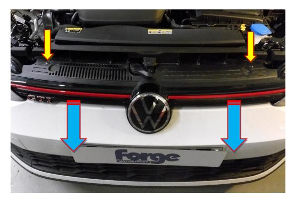
3. Un-plug the ACC wiring loom attached to the centre of the grill.
