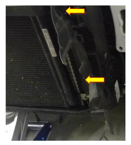
24. Push in the locking tabs securing the air conditioning condenser, lift the unit upwards to release it from the radiator pack.
