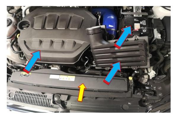
7. Using a T25 Torx and drive remove the x4 M5 fasteners on the top edge of the bumper cover.
