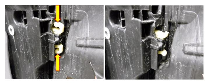
**26**. Remove X4 foam rubbing strips as these will no longer be needed.
