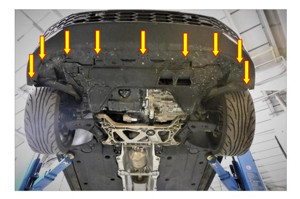
**11**. Using a T25 torx and drive remove the x8 M5 fasteners attaching the undertray to the vehicle.
