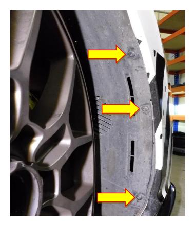
9. Peel back the top of the arch liner to reveal the M5 fastener on each side and use a T25 Torx and drive to remove them.
