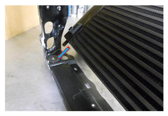
**31**. Take the X2 machined clamps and using a 5mm Allen key loosely attach X2 M6 fasteners to the intercooler.
