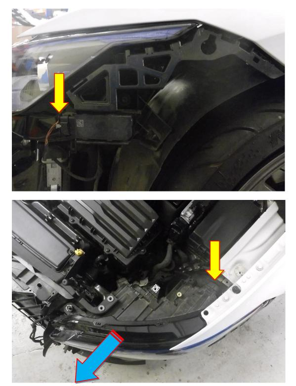
**16**. From underneath the vehicle, using a 7mm socket and ratchet loosen both hose clamps and remove the boost pipes attached to the intercooler.
