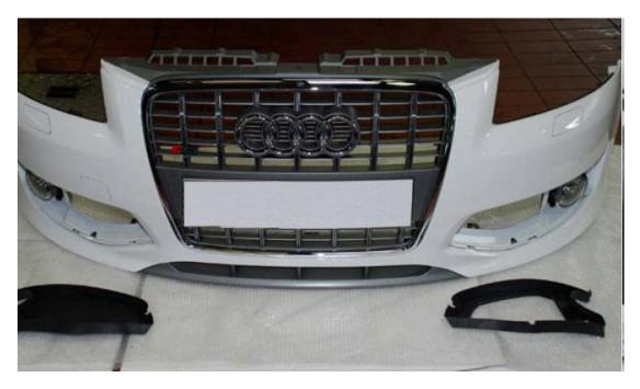
The lower grills need to be removed from the front panel on both sides. Then the grill backing panels are removed, these will not be refitted. Mark the front panel as shown if this picture.
