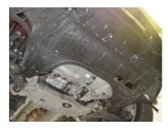
3/ Remove the 8x T25 screws in order to remove the complete engine under tray.
