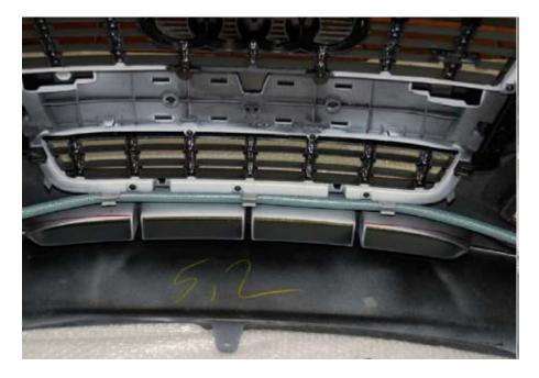
Again remove with a jig saw or open saw blade on both sides. Once the front panel has been trimmed refit it too the vehicle. If necessary trim more from any areas as required. Refit the undertray and bumper in reverse of removal. The lower outer grilles may require a small amount of trimming to be able to fit them back in to place.
