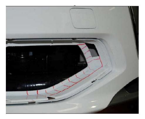
Then cut the panel to allow clearance for the hoses. This is required both sides.
