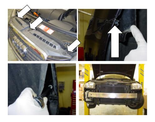
2) Remove the 2x radiator air deflectors. These are fixed with a single T20 screw in each. These will not be refitted later.
