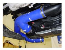
8/ Before the front panel can be refitted it is necessary to trim the panel to increase clearance.
