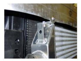
5/ Remove the horns from their brackets, now remove each bracket from the car and refit the horns as per the pictures below with the new brackets supplied so they are now sited higher. This is to allow the new hoses a free routing below the horns.
