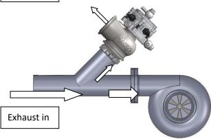
Angled mounting is good for flow into the wastegate, and should be the minimum you aim for in your installation
