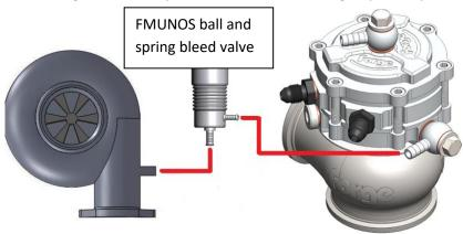
If you are running an electronic boost controller, then please follow the guidelines laid out in the boost controller instructions *based on an external wastegate setup*. A typical installation is laid out below, where the boost controller solenoid sits in a line teed off the lower port of the wastegate, going to the upper port of the wastegate to vary the resistance above the piston, but please double check for your specific boost controller.
