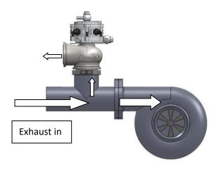
With the wastegate at 90 degrees to the flow of exhaust gas, the boost control will be compromised.
