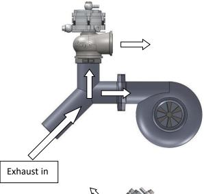
Symmetrical mounting of the turbo and wastegate is excellent for boost control, but not always possible upon installation due to space constraints
