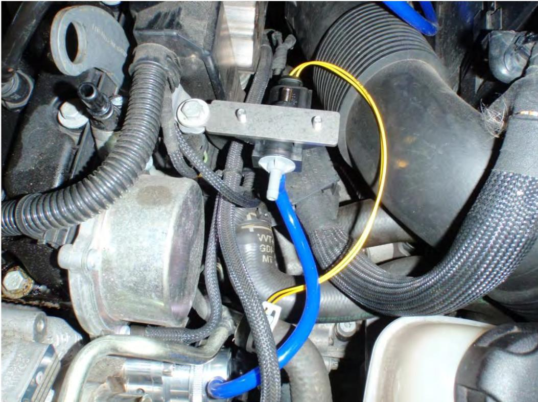
8. Route the vacuum hose from step 3 around the engine bay and into the horizontal nipple on the solenoid as shown. Use the supplied small cable ties to secure the vacuum hose to all of the nipples (DV, MAP boss, solenoid) and around the engine bay.
