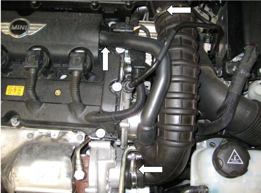
2. Remove the airbox by undoing the single bolt on the left hand side, then pulling it upwards to remove it from the rubber grommets that hold it to the top of the inlet manifold, giving you access to the cold air feed that simply pulls off the right hand side.
