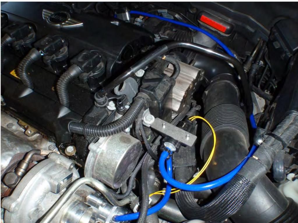
9. Refit the airbox removed in step 2 making sure that you don't pinch the silicon vacuum hose underneath it, and the hoses removed in step 1. You could take this opportunity to upgrade the Forge inlet pipes at the same time (FMR56IND for Mini, FMINL207 for Peugeot).
