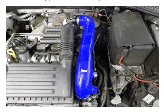
13. Fit the new Forge Motorsport dump valve into the hose and tighten the hose clamp that holds it in position. Fit supplied blanking plug to second hose spout if it is not required.
