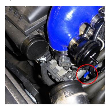
14. Locate the manifold vacuum pipe (area circled in previous picture) and disconnect. Fit supplied vacuum T in between manifold and disconnected pipe and use E-clip to secure in place.
