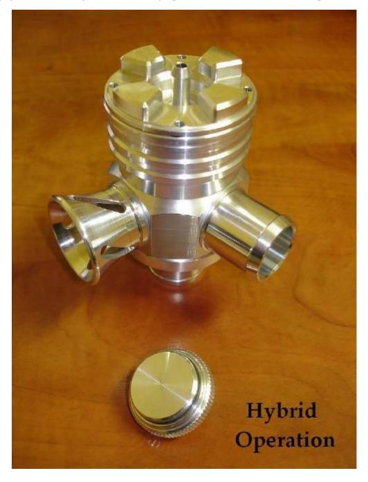
If the user chooses to setup the valve in a 100% recirculating configuration, the discharge horn will need to be removed (unscrewed) and replaced with the blanking plug on the body of the valve. Nothing else will need to be changed for this configuration of the valve. Please see below:
