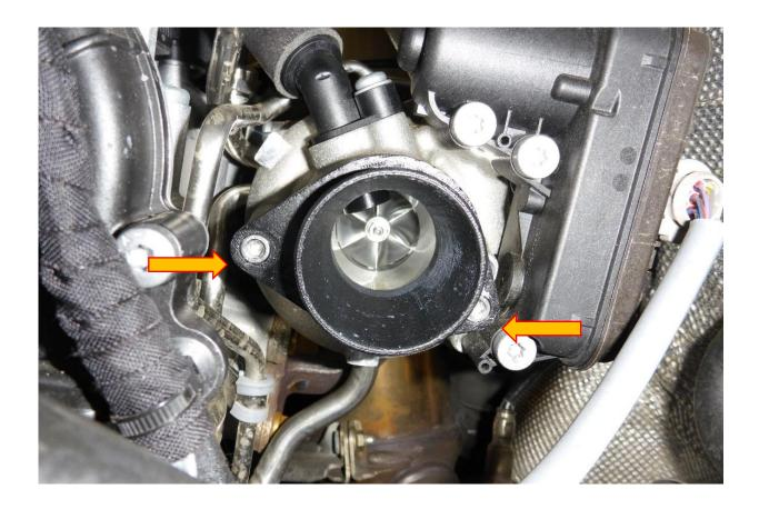
8. Fit the Forge silicone intake hose to the turbo adaptor, using a 7mm socket and rachet or a flat bladed screwdriver fit the 50-70 hose clamp to secure it in place.
