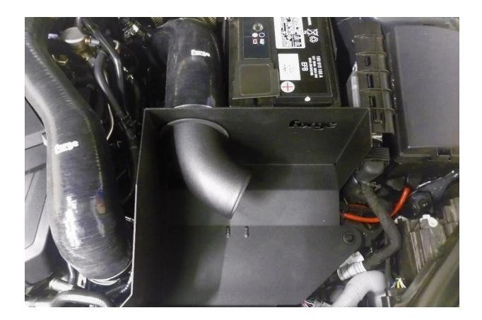
12. Fit the Forge filter onto the end of the alloy intake pipe and secure it into place with the remaining 70-90mm hose clamp. Angle the filter so that it has between 10mm-15Mmm clearance from the bottom the filter tray, then tighten the other hose clamp fitted in step 11. Use a 7mm socket and rachet or flat blade screwdriver to tighten the hose clamps.
