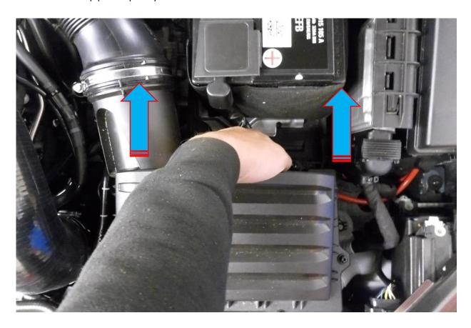
3. Release the two Norma fittings attaching the breather hoses to the turbo elbow. If your vehicle is not equipped with this system ignore the rest of the breather system steps.
