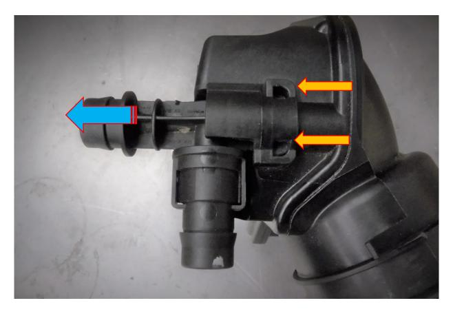
6. With the breather adaptor now removed, take the Forge Motorsport billet breather adaptor, and push it onto the end of breather adaptor with the green O ring. There is location marker on the billet adaptor which must be lined up with the plastic moulded line as shown in the picture below. Use the U clip supplied to secure the billet adaptor in place.
