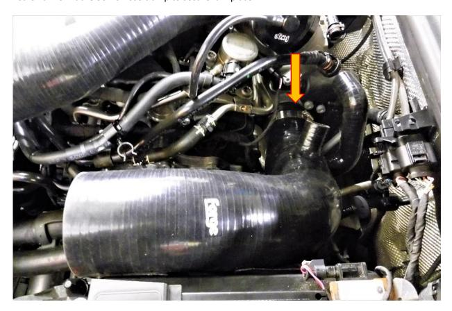
9. Take the breather adaptor and insert the billet end into the spout coming from the Forge intake hose. Secure it in place with the supplied 16-27 hose clamp, then re fit both breathers. If you are not installing our recirculation valve (FMDV30) install the supplied alloy blanking plug and secure it with the other 16-27 hose clamp.
