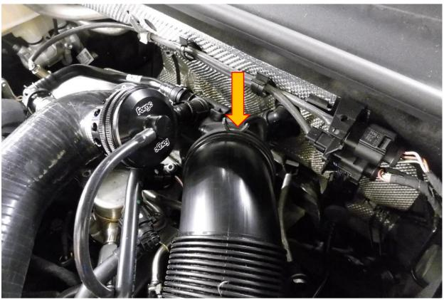
2. Pull the air box upwards sharply to release it from its rubber mounting points and remove it and the attached intake pipe completely from the vehicle.
