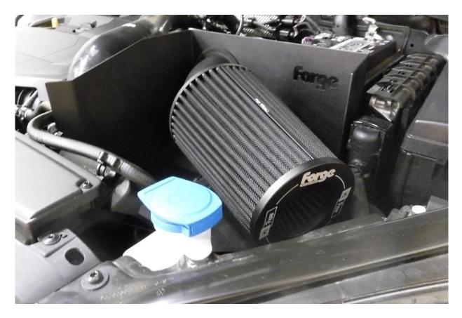
On certain vehicles with the washer spout is in the location below, you may have to position the air filter further down the alloy intake pipe.
